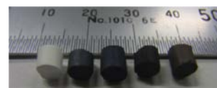
Figure 1. Photograph of anatase \text{TiO}_2 , \text{Ti}_6\text{O}_{11} , \text{Ti}_4\text{O}_7 , \text{Ti}_3\text{O}_5 , and \text{Ti}_2\text{O}_3 monoliths (from left to right).
